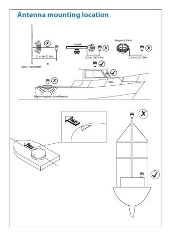
Just like any other GPS antenna, Point-1 should be mounted where it has a clear, unobstructed view of the sky in order to ensure quality signals from the satellites.
